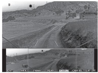
The pan position indicator on the bottom half of the display indicates what portion of the scene is displayed on the upper part of the display.
