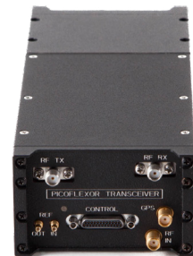
PicoFlexor Transceiver with AEP Module for application development
