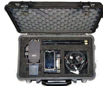
Custom packaged RF Survey System in a 1510 Pelican Case
