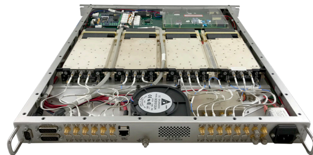
When the top panel is removed, four Sparrow tuners are shown installed into the equipment frame
