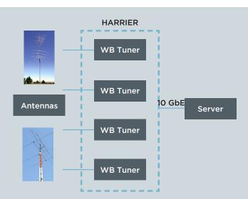
Networked VLF/HF architecture. The Harrier tuner can be coupled with a standard server in a networked environment for flexible data distribution.
